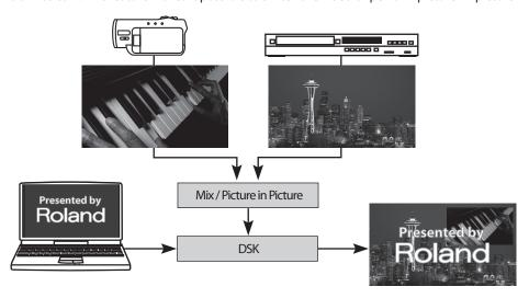
By default, the video on channel 4 is displayed in the foreground of DSK compositing. If you are using the unit with the default setting, input the logos and text to channel 4. To change the setting, refer to "Menu Operations and Menu List" (p. 45). Also, the extraction color for DSK compositing is set to black by default. You can use the menus to change this as well.
