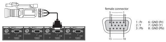
To assign component input to channel 2, go to [A-BUS/PGM] and press [2], then press the [RGB/COMPONENT] button. When the V-40HD detects the component input, the [INPUT STATUS] indicator of the channel 2 lights up.
