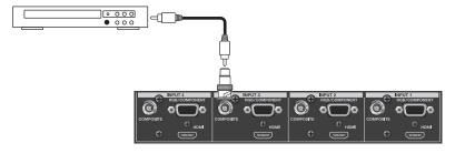
To assign composite input to channel 3, go to [A-BUS/PGM] and press [3], then press the [COMPOSITE] button. When the V-40HD detects the composite input, the [INPUT STATUS] indicator of the channel 3 lights up.
