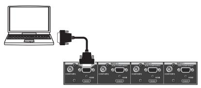
To assign RGB input to channel 4, go to [A-BUS/PGM] and press [4], then press the [RGB/COMPONENT] button. When the V-40HD detects the RGB input, the [INPUT STATUS] indicator of the channel 4 lights up.
