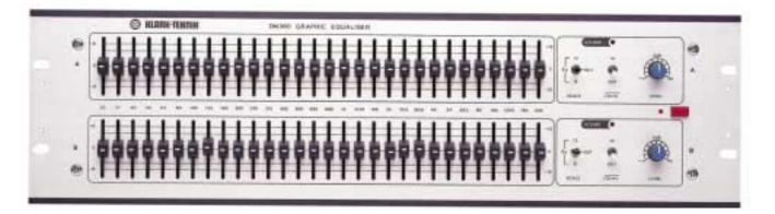
The Klark Teknik DN360 is a dual channel, 30 band equaliser offering 12dB of cut or boost in 1/3 octave steps between the frequencies of 25Hz and 20 kHz.
