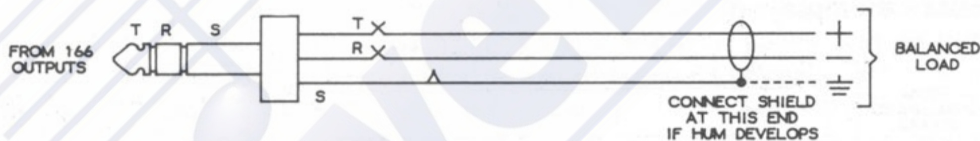
Figure 4: Balanced ins and outs, dual-conductor shielded cable, stereo plug
