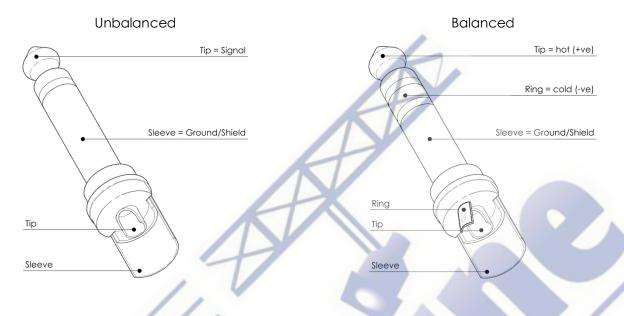
For these applications the unit provides 1/4" TRS and XLR connectors to easily interface with most professional audio devices. Follow the configuration examples below for your particular connection.
